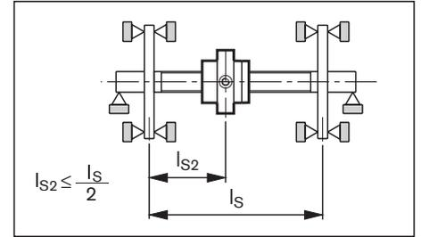
$$R_{S2} = 165 \cdot \frac{(d_0 - 0,71 \cdot D_w)^2}{l_{S2}} \cdot \frac{l_S}{l_S - l_{S2}} \quad (\text{N}/\mu\text{m}) \quad 18$$
