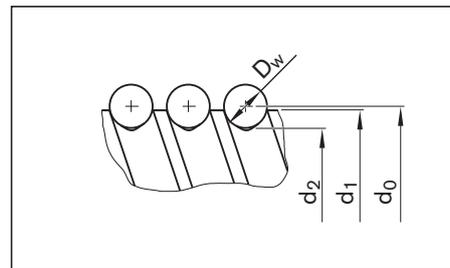
$$R_{S1} = 165 \cdot \frac{(d_0 - 0,71 \cdot D_w)^2}{l_{S1}} \quad (\text{N}/\mu\text{m}) \quad 17$$
