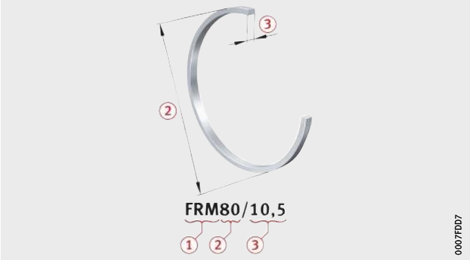
Figure 9 Designation structure of locating rings, example
